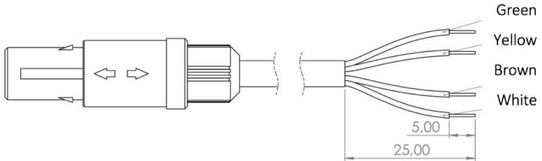
Figure 7: Electrical connection of cables to the measuring instrument
