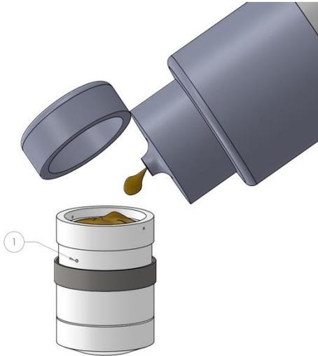
Figure 4: Cap filling phase with gel electrolyte.
