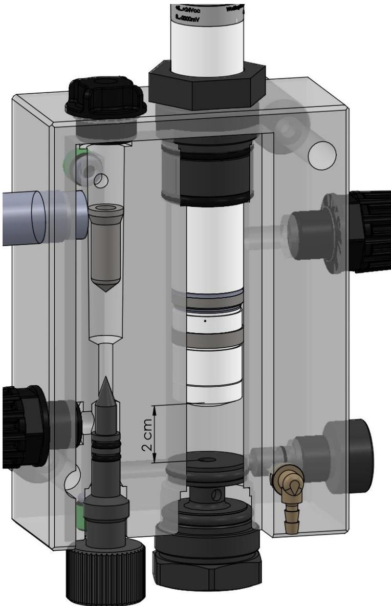
Figure 6: installation of the probe in a probe holder, where the optimal operating distance is shown
