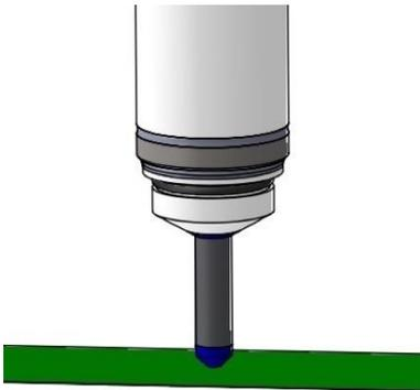
Figure 10: Cleaning the working electrode with abrasive paper
