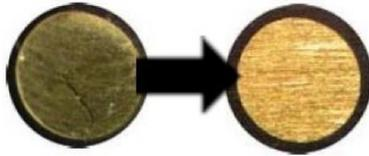
Figure 9: Working electrode before and after cleaning
