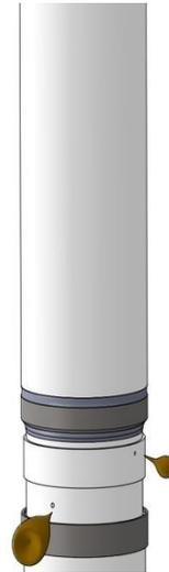
Figure 5: Assembly phase of the cap on the probe.
