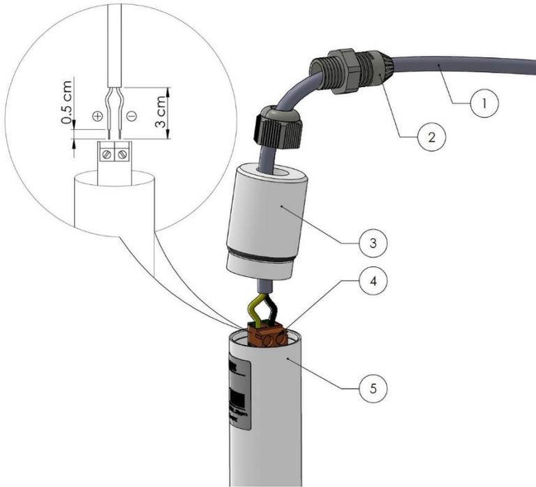
Figure 8: Electrical installation for probes with two-wire current output
